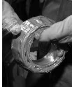
Fig. 23. Grease can easily be packed by hand.
